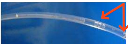
Figure 6 HPFA+ Tubing Showing Broken Air Gap
