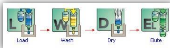
Figure 3. TRILUTION® LH THC Solid Phase Extraction Method Using the Gilson GX-274 ASPEC™ System
