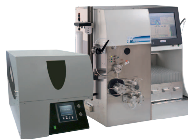
Figure 3 CPC 250 with PLC 2250 Purification System
