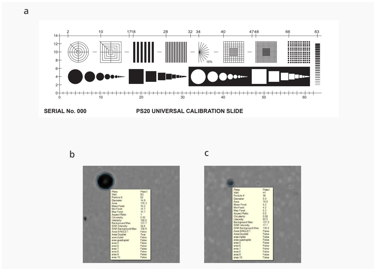
**Figure 5:** Sizing with the Aura system. (A) Calibration with ASTM Microscope Slide. Particle size verification with (B) 15 µm and (C) 5 µm polystyrene bead standards as shown in the captured images from the Aura Particle Vue software tooltip.
