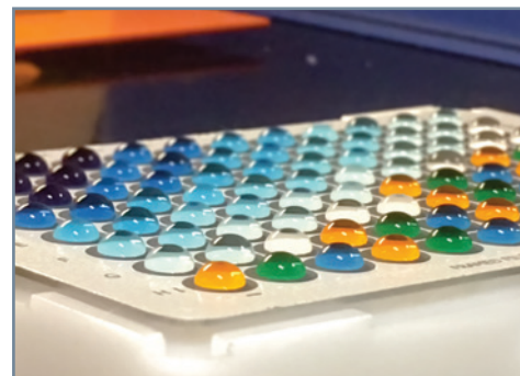
Proprietary 96-well filter plate laid out to demonstrate a complex multi-condition experiment
