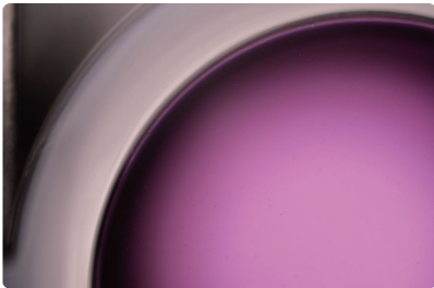
Conventional image of a well with a broad and dark edge affecting cell recognition.
