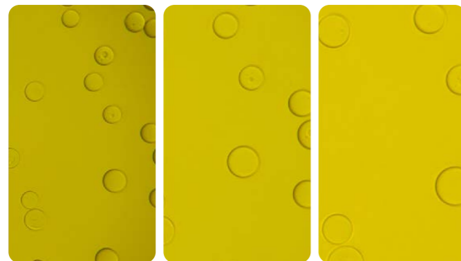
From left to right: Cross-linked Agarose particles (20 \mu\text{m} to 50 \mu\text{m} ); 5.0x, 6.6x, and 8.0x magnification; Cell Counting BioApp
